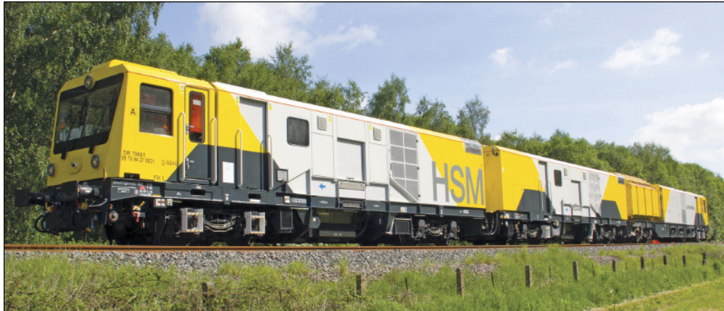
Above: The HSM high-speed milling train during trials at Network Rail's RIDC Tuxford.
