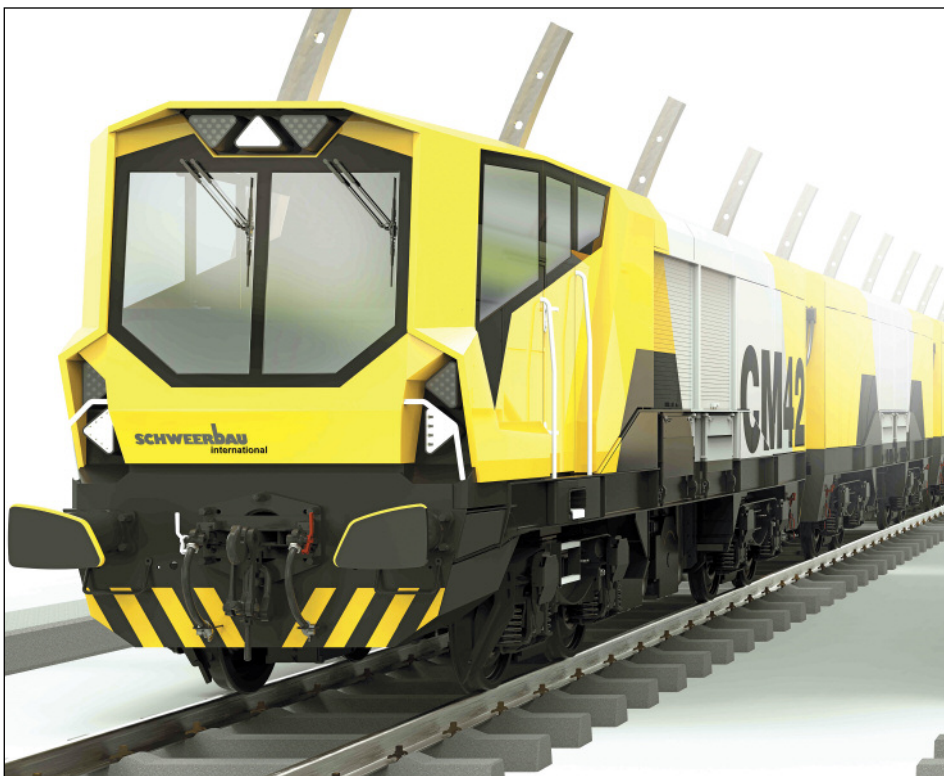
Below: The CM series will be the next generation of rail milling trains from Schwebbau.
