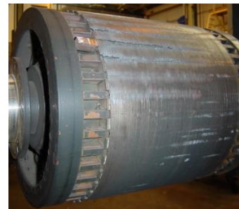
DMKT 52/24 Traction Motor Rotor with Failed Rotor Bars.
