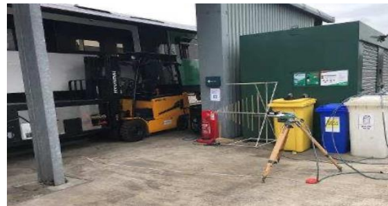
Figure 2 - Radiated Emissions Testing of DGS at Vivarail
