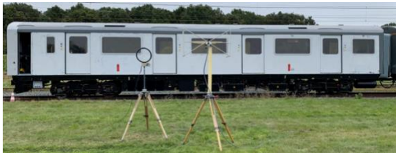
Figure 3: Radiated Emissions Testing of the COP26 Battery Train
