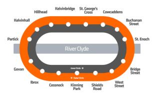
Glasgow's Subway comprises a four-foot gauge double track in a circular 10.5km tunnel. First opened in 1896, it is the world's third oldest underground railway after London and Budapest. The modernisation marks the first major enhancement of the subway for 40 years and will link to other transport infrastructure improvements across Glasgow to contribute to the city's regeneration programme.
