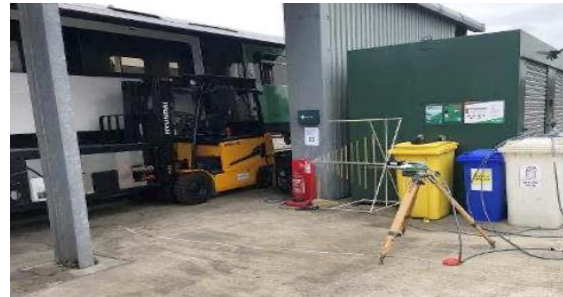
Figure 2 - Radiated Emissions Testing of DGS at Vivarail
