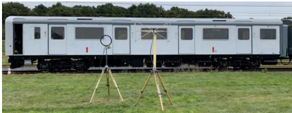
Radiated Emissions Testing of the COP26 Battery Train
