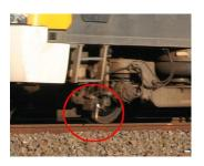
Tripcock train protection is about to be decommissioned and replaced with Train Protection Warning System (TPWS). On top of the TPWS, the ETCS Level 2 is going to be implemented.
